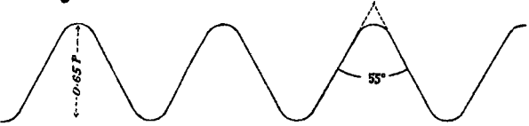
Fig. III. Form of Thread introduced Mr. Whitworth.
